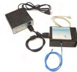
Sol Spectrometer, Power Supply and Cables
